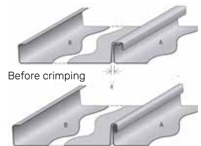
After crimping (double crimped standing seam)
